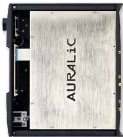
ABOVE: Hidden within the alloy chassis, and screening the circuitry within, is a branded nickel-plated copper enclosure
