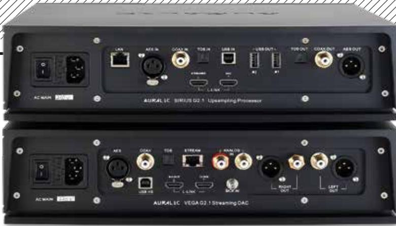
**ABOVE:** Sirius G2.1 [top] includes LAN control input plus digital in/out on coax, Toslink and AES (DSD64/192kHz) plus USB and L-Link in/out (DSD512/384kHz) on HDMI. Vega G2.1 [bottom] has complementary digital inputs, an external clock input, analogue line inputs and fixed/variable analogue outputs on RCA and balanced XLRs
