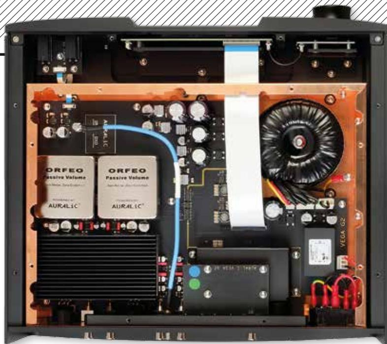
**ABOVE:** The Vega 2.1's linear PSU [top right] feeds the screened-off DACs [top left], ladder volume controls [centre left] and 'Class A Orfeo Output modules' [heatsink, bottom left]
